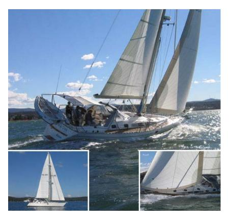
The sail combination and setup is designed for good light air to heavy weather performance. Having a SA/Displacement Ratio of 17 puts her into the cruiser/racer category. The 122% radial cut overlapping genoa is designed to be efficient from 5-20 knot wind range while the self tacking staysail suits the 25-45 knot wind range. The radial cut main can be electrically furled to any size making it suitable from 5 to 45 knot wind range.
